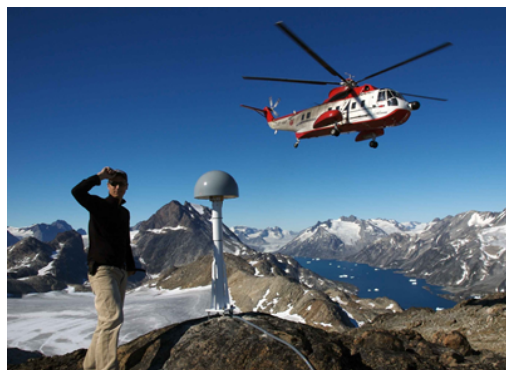
Abel Brown from the Ohio State University awaiting pick-up after installing GPS station TIMM on Timmiariit Island in southeast Greenland.
