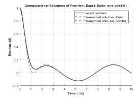
Figure 5: The MATLAB<sup>®</sup> plots for position x(t): Exact, Euler, and ode45().
