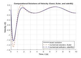
Figure 6: The MATLAB<sup>®</sup> plots for velocity v(t): Exact, Euler, and ode45().
