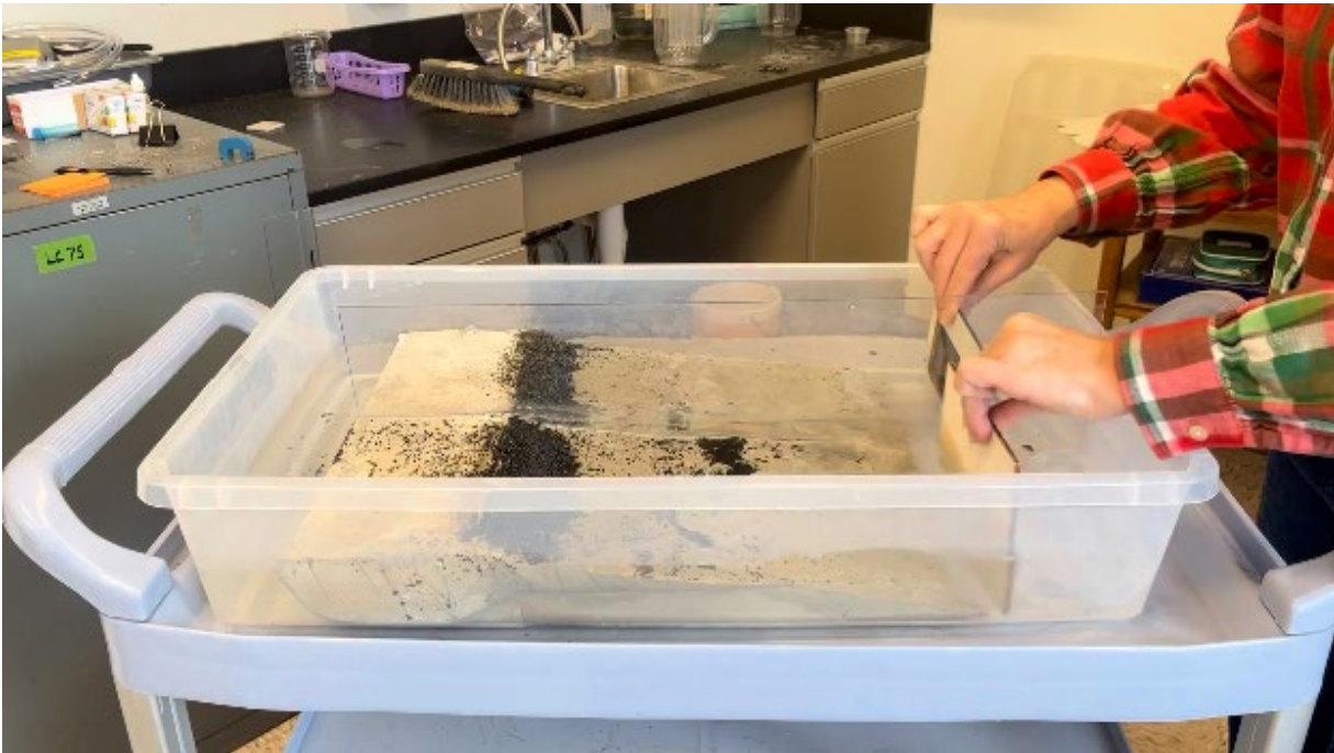
Figure 2. This is the physical model to demonstrate the effect of small vs large waves. The tank is separated with a Plexiglas sheet in the center. The sediment is uniform in size on both sides of the model. The waves are created with two paddles- one is solid and the other has screen in the center. The paddle with screen will make smaller waves. The sediment with larger waves will mobilize first.
