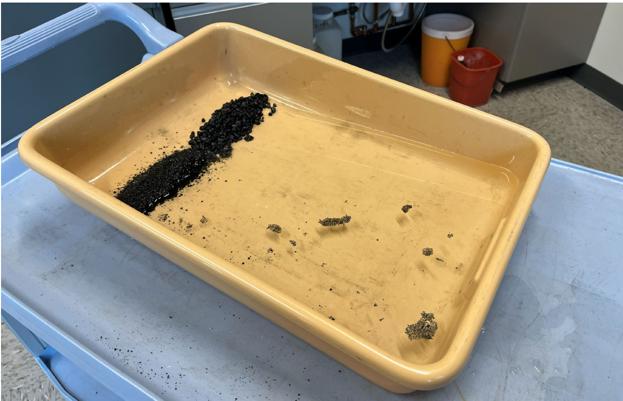
Figure 3. This is the physical model to demonstrate the effect of grain size on shoreline stability. The model is a plastic tray propped up on one end with a 2x4 to create a slope. There are 2 sediment sizes used. The sediment closer to the camera is finer than the sediment on the far side. Both sediments were aquarium gravel purchased at a pet store. The store sold the gravel in 2 sizes. Waves are created in the deep end with a block of wood.
