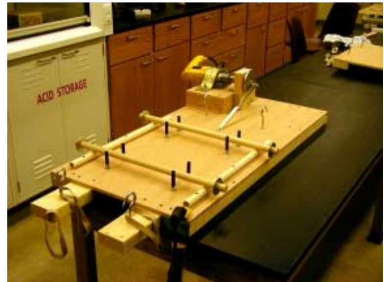
Figure 4. Top view of table showing locations of wooden dowels. Note washers attached to dowels.
