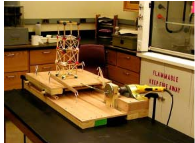
Figure 15. Assembled shake table with Popsicle stick building. Note c-clamp securing the table to the table upon which it rests.
