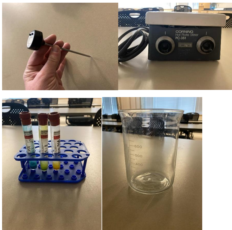
Figure 3. Material needed for the lab at each station: Digital thermometer, a hot plate, a tube holder with three test tubes, and a large beaker. Additional material for the mixture preparation: scale, weight paper, hour glass, and spatula.
