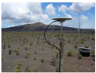
GPS station KAMO, with Pu'u ' $\overline{O}$ 'ō in the background. The GPS antenna is in the foreground, with the solar panel, electronic box, and telemetry mast, and telemetry antennas at right. (2007/08/10)
