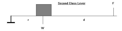
A smaller effort can be used to advantage over a larger weight. An example of this lever is a wheelbarrow.
