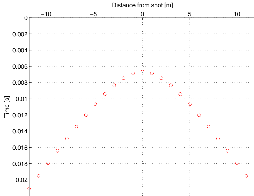
Figure 2: Arrival times of the reflected wave with wave velocity 600 m/s, reflector depth 2 m and geophone spacing 1 m.
