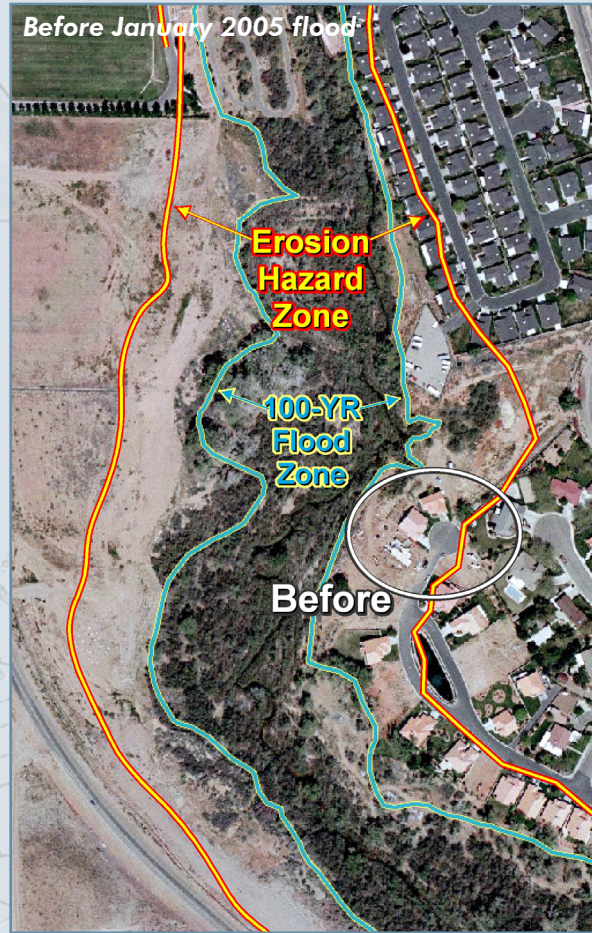
The January 2005 flood event in St. George, Utah. Aerial shot of Erosion Hazard Zone compared to 100-year floodplain.
