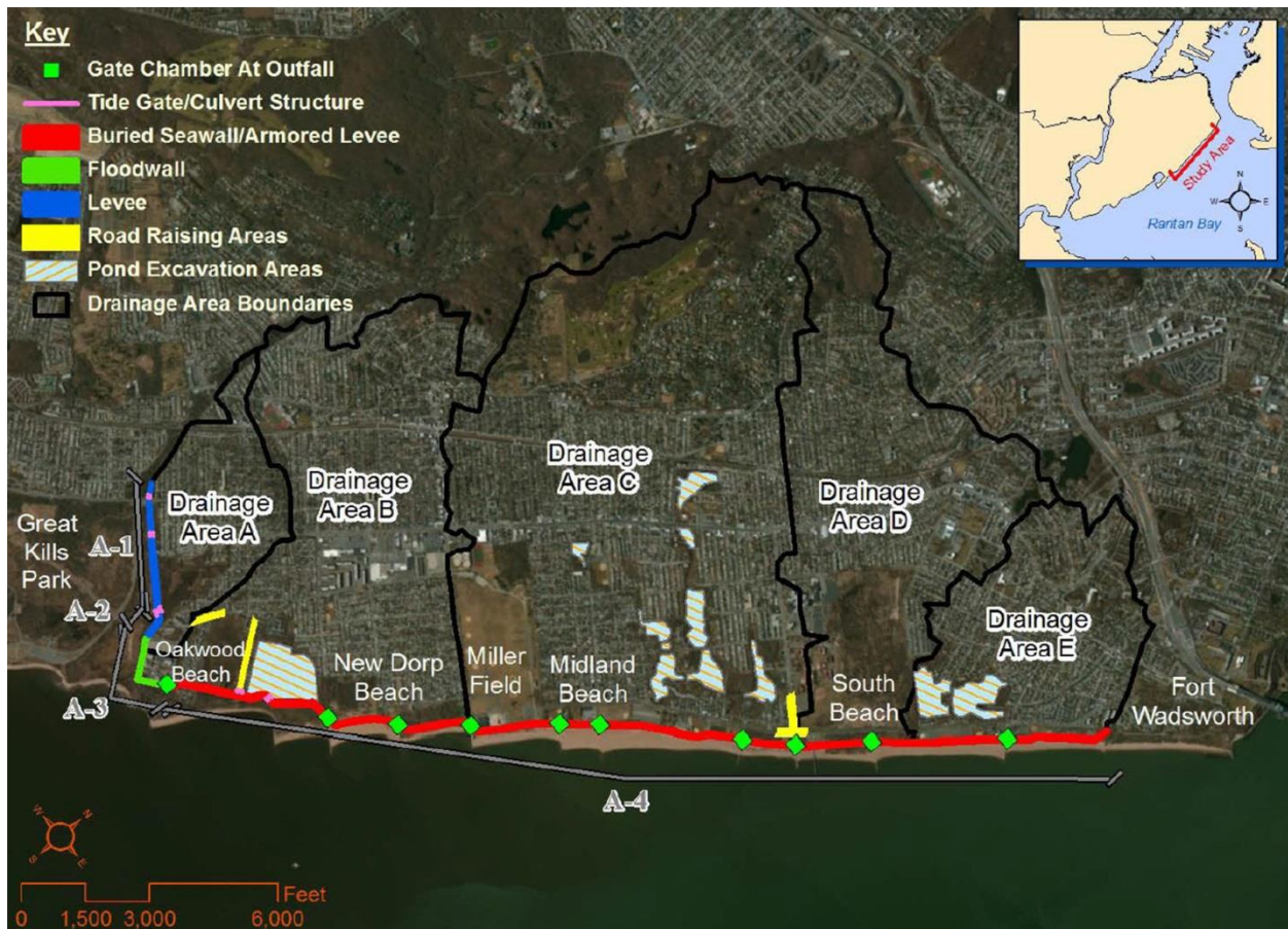
Figure 9 U.S. Army Corps of Engineers proposal for a Sea Wall with a boardwalk on top.
