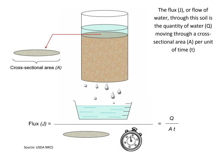
In the "How Full is Full" activity, we are looking at flux as a reflection of the permeability of our soil samples. The formula above can be used to calculate the actual flux.
