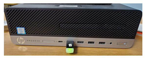
• Insert the Geogiga Dongle into a USB port of the computer.
