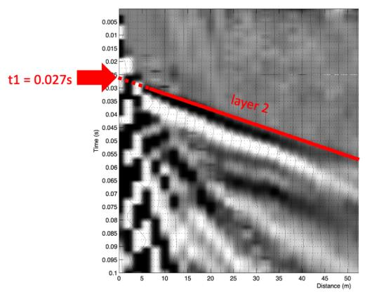
Based on the slope of the layer 2 refraction arrivals that you already identified in step #1, project this line back to the time axis, as shown by the dashed line above. The "t-intercept" will be t1 that we need for the next calculation.
