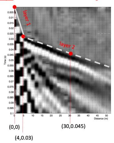
Step 2: extract rise-over-run values from the image on the slope of layer 1 and layer 2
