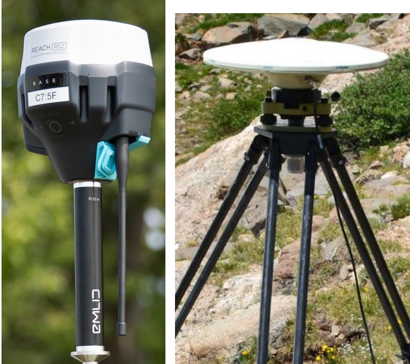
Figure 2: (Left) Emlid Reach RS2 antenna/receiver combination (Photo: Andy Moore). It contains a LoRa radio and is designed to be self-contained. (Right) Trimble Zephyr geodetic antenna mounted on a tripod and connected to an external receiver via a port on the bottom of the saucer. (Photo: Ian Lauer)
