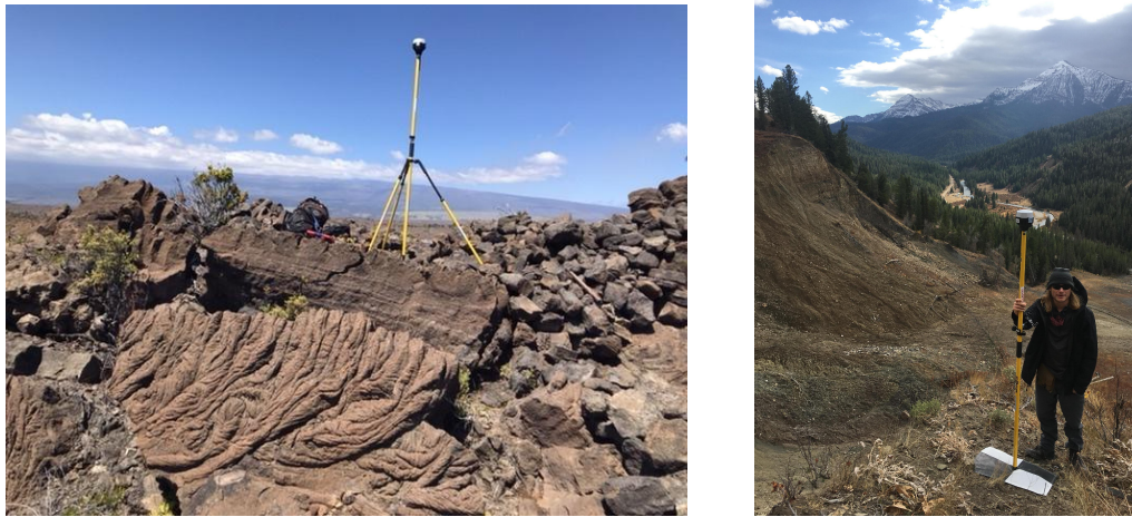
Figure 1. An example of a Real-Time Kinematic (RTK) base station (left) and rover (right). Many options are available for rover mounts including poles, bipods, and backpacks (shown). A PPK setup is essentially the same, minus the radio link. (Source: Steve Lundblad and Benjamin Crosby)
