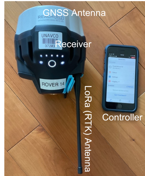
Figure 6. An example of the main components on Emlid Reach RS2 PPK or RTK rover. GNSS antenna, receiver, and LoRa antenna are together. The controller is a phone/tablet app. (Source: Beth Pratt-Sitaula)
