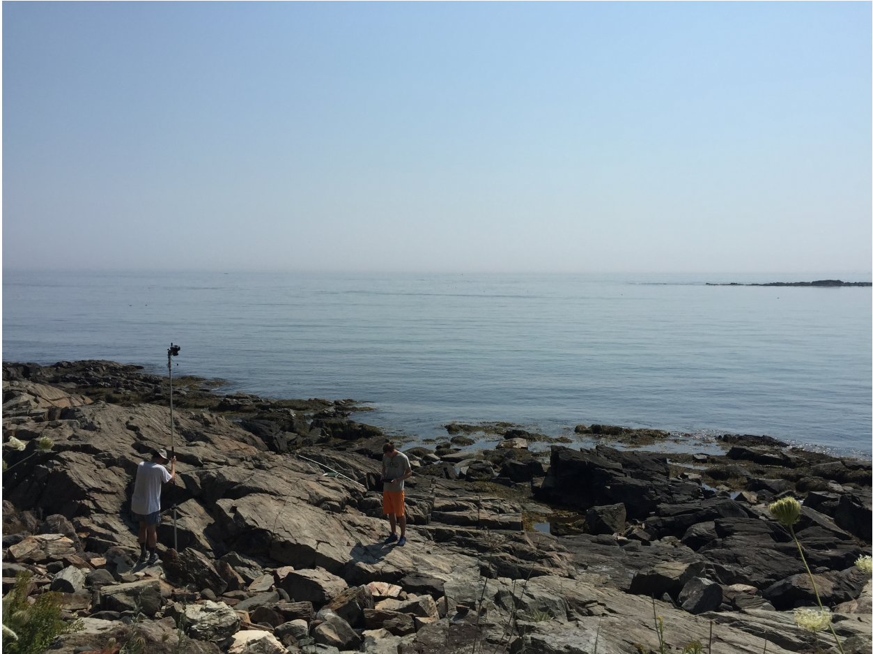
Figure 3. Pole aerial photography (PAP) platform. This platform requires a long, telescopic pole to elevate your camera for the purpose of shooting down on the area of interest or to reach higher on an outcrop. The camera will need to take photographs at certain intervals and can be accomplished through time-lapse, continuous, or remote-controlled shooting. Many cameras (particularly newer DSLR have apps available that allow the camera to be controlled by a smart phone). These researchers are photographing a series of small, melt-bearing strike slip faults within the nearly horizontal outcrops. Photo: Katherine Shervais.
