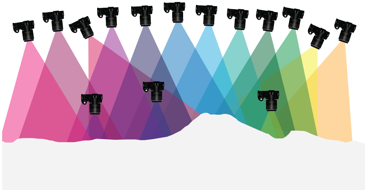
Figure 12. Take photos converging on the feature, at multiple distances and angles.
