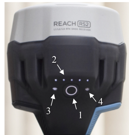
Figure 1. Image of the Emlid Reach RS2 receiver. (1) power button, (2) battery status, (3) Wi-Fi status (4) RTK status
