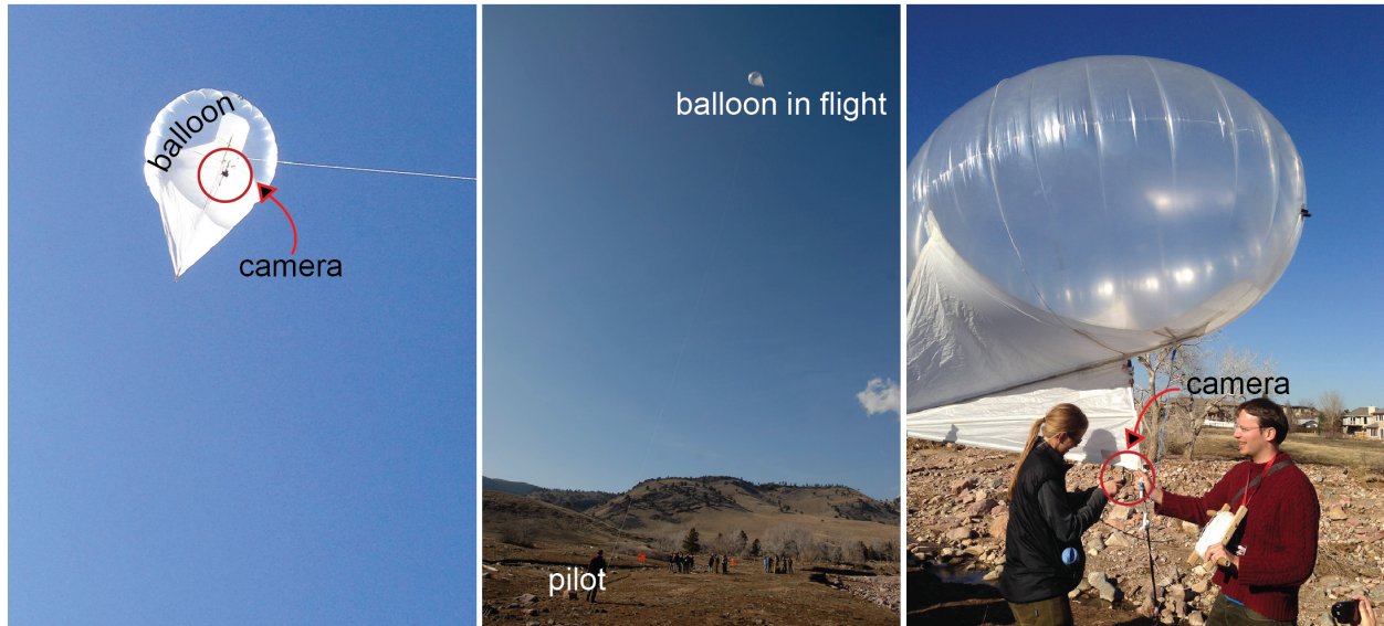
Figure 4. Balloon platform. The photo on the left shows the position of the camera while the balloon is in flight. The center photo shows the position of the balloon relative to the pilot while in flight; the photo on the right shows the more detail of the camera setup. Because of the picavet setup, the camera is oriented directly at the ground. See Figure 5 for a schematic of how this works. Photos: 2014 UNAVCO Science Workshop, Beth Bartel and Linda Rowan.
