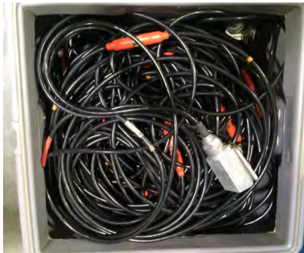
Figure 13. Proper Spaghetti-style method for storing Geode cables
