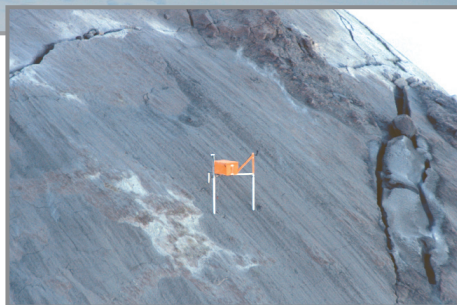
View of north side of the new lava dome from a location immediately south of 1980-1986 lava dome. Circle shows the location of an instrument station on the dome. Inset shows the instrument station, a "tilt-leg spider" package named CDAN, on top of the north-face of the new dome. This station housed a GPS unit and a seismometer until it was destroyed by an explosion on January 16, 2005, 36-hours after placement. (USGS photos, January 14, 2005).
