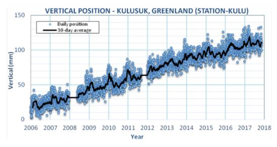
Figure 1. Vertical GPS data from station KULU near Helheim Glacier in Greenland from the beginning of January 2006 to the end of December 2017.
