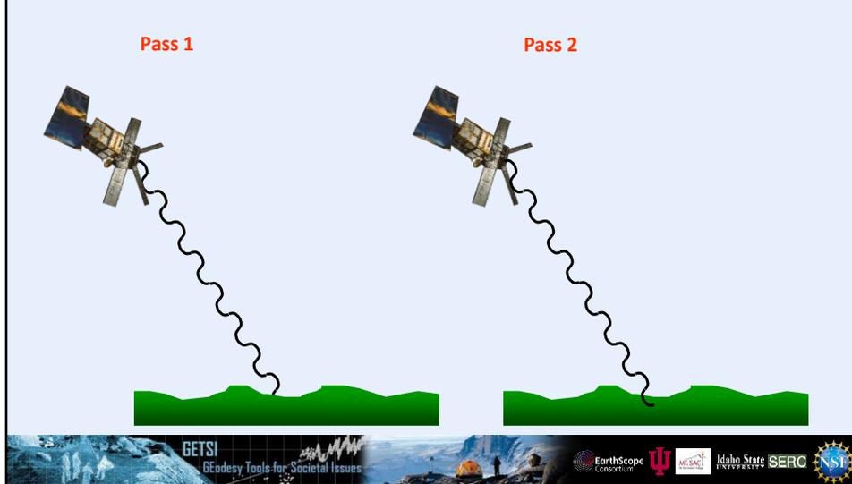
. . . So what we do is compare (difference) the phase from two different passes of the same satellite over the same point on the ground. Assuming that we can correct for the position of the satellite (and we can), then any difference in phase between the two passes must be related to a change in distance between the satellite and the ground (i.e. a movement of the ground).
