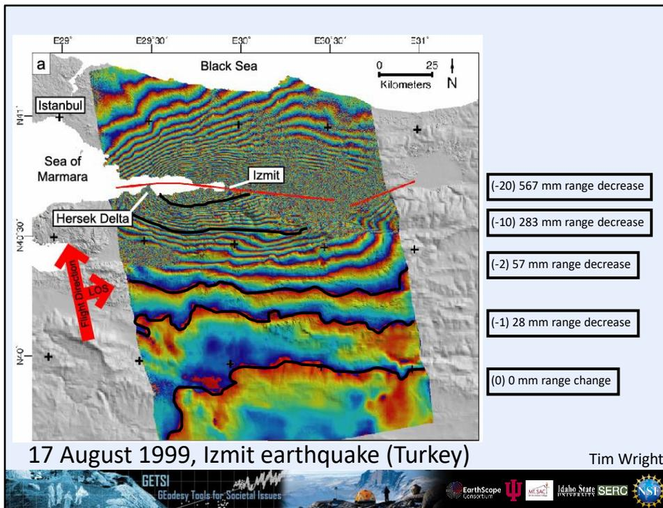
How to interpret an interferogram? To begin we have to be sure of the sign convention of the deformation signal. Here each colored “fringe” from blue to yellow to red represents a movement of the ground toward the satellite of 28.3 mm in the line-of-sight direction (this is often described as a decrease in the range—that is to say, the distance—between the satellite and the ground).
