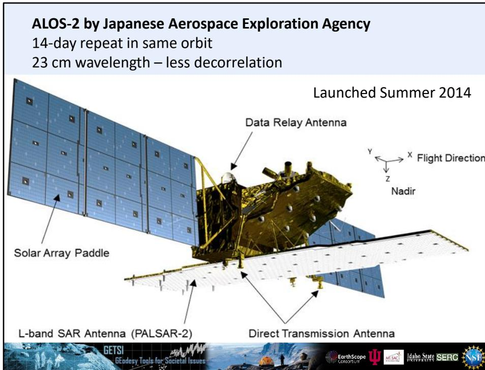
Not to be outdone, the Japanese Aerospace Agency (JAXA) has launched a SAR satellite, ALOS-2, that is designed to be effective in vegetated areas. Using a 23 cm wavelength (rather than the ~6 cm wavelength of Sentinel-1), it should be impervious to small changes in vegetation, which is important for imaging deformation in heavily forested Japan.
