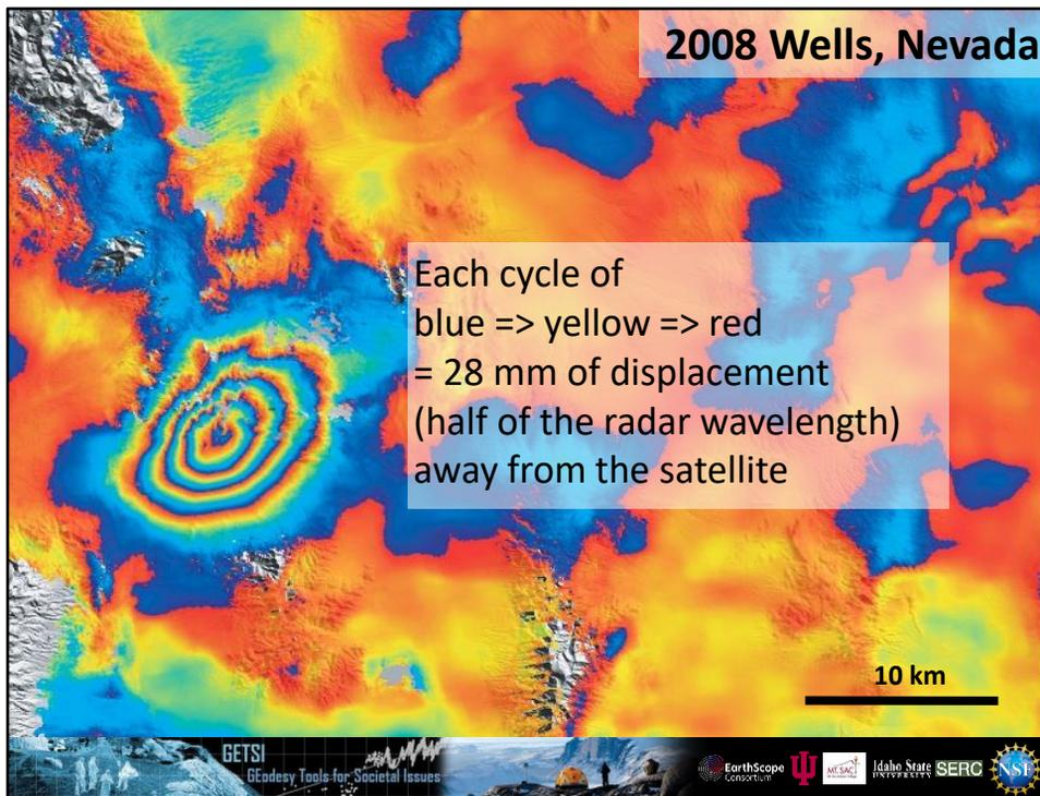
Here is another earthquake interferogram, from the 2008 Wells, Nevada earthquake. In this case, each cycle of blue to yellow to red represents an increase in distance (a range increase) of 28 mm between the satellite and the ground. [Note that there is no standard convention for the color scheme of interferograms!]
