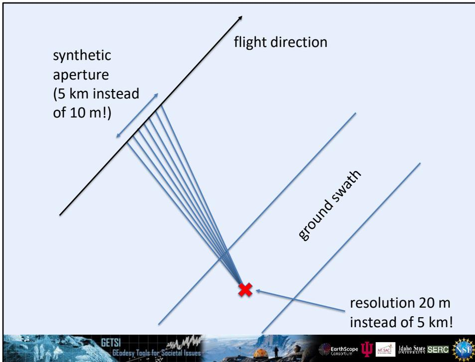
When we process the data, we can integrate all the images that would have covered the same point on the ground to effectively pretend that the radar antenna had an aperture of several kilometers length. This “synthetic aperture” idea is what allows us to make high-resolution images of the ground using satellite-borne radar.
