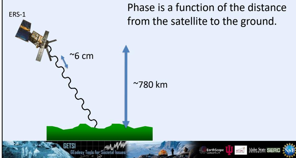
Recall that one wavelength of path length is equivalent to  $2\pi$  of phase. Given that radar satellites orbit at several hundred km of elevation, it is not feasible to count the number of phase cycles for a single image . . .
