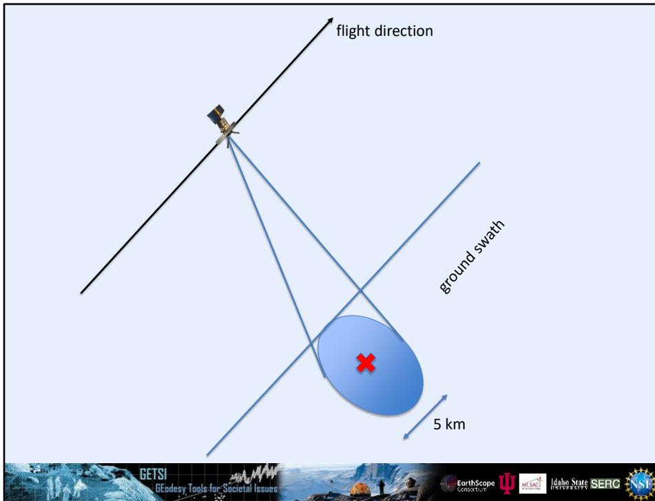
The radar antenna is mounted on the right side of the satellite (in SAR-speak, we say that the radar “looks to the right”). The idea behind this is that we can know for certain which direction any backscattered radar is coming from (which would not be possible if the radar was pointing vertically down).
