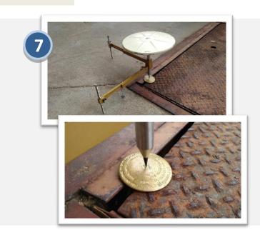
A metal tag will be attached to one of the horizontal arms. Stamped on the tag is the antenna height, or the distance from the tip of the center rod point to the base of the antenna in millimeters. These values will be around 250 mm but will vary slightly and are measured annually. The antenna height value must be recorded and is an important component of data processing.
