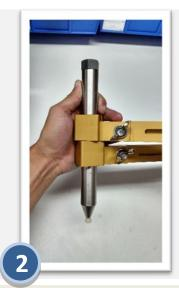
To open the arms, loosen the two wing bolts highlighted in the photo above. Try to arrange the arms at an approximately 90° angle to one another for maximum stability. Please retain the protective plastic caps on the top and bottom of the center post for use in transport.
