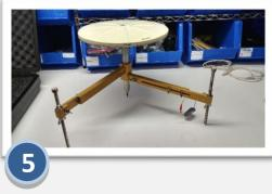
When your center post with point is installed over the correct location, securely thread on the bi-directional level (4a). Use the bottom wing nut on the leveling rods (4b) to adjust the angle of the horizontal arms. When the bubble of the bi-directional level is centered in the glass, set the leveling rod by tightening down the top wing nut (4c).
