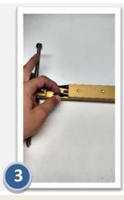
Inside one of the horizontal arms, you will find the precision points to be used on the central rod. These are threaded into the arms and should come out fairly easily. Please take care with the points as bending or dulling will change the antenna height.
