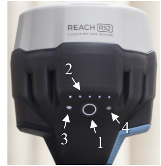
Figure 1. Image of the Emlid Reach receiver. (1) power button, (2) battery status LEDs, (3) WiFi status, (4) RTK status
