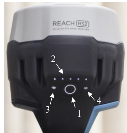
Figure 1. Image of the Emlid Reach RS2 receiver. (1) power button, (2) battery status, (3) WiFi status (4) RTK status. Steady white WiFi status means receiver is in Hotspot mode. Blue it is connected to a local WiFi network.
