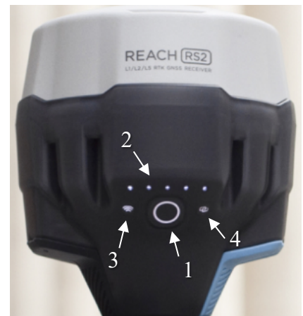
Figure 1. Image of the Emlid Reach RS2 receiver. (1) power button, (2) battery status, (3) WiFi status (4) RTK status. Steady blue WiFi status means receiver is in Hotspot mode. White it is connected to a local WiFi network.
