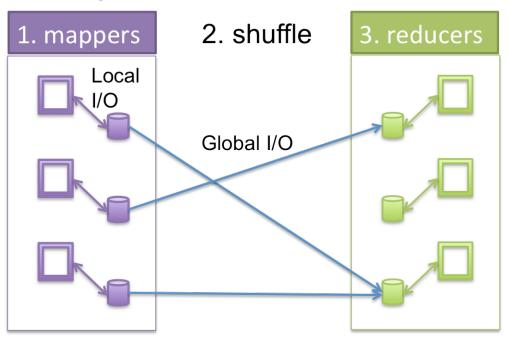
Stages are controlled by functions: mapper(), reducer()
