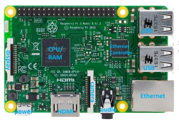
Single Board Computer Quad-Core Multicore CPU 1 GB RAM \$35.00
