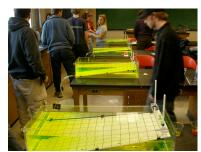
Engineering curriculum, students study the processes that are active on the surface of the Earth. In this lab we ask the question: "What happens when a dense fluid flows down a slope, underneath less-dense
