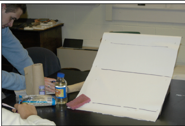
Figure 1A. Oblique frontal view of a viscosity ramp. Lines are for reference so that students can calculate syrup flow velocities. The material covering the surface is padded vinyl shelf paper.
