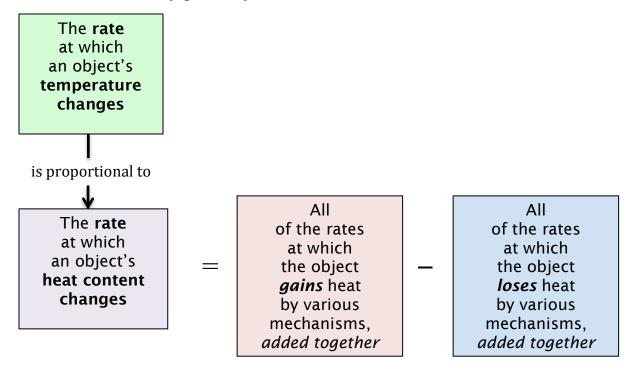
We could apply this law to the earth's surface. Moreover, if we suppose that the surface *gains* heat only by absorbing solar radiation, and it doesn't *lose* heat by *any* mechanism, then the Law of Conservation of Energy applied to the earth's surface would be simply:
