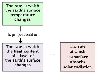
Using this relationship, if we know how fast the surface absorbs solar radiation, then we can calculate how fast the surface temperature changes. From that, we can estimate what the temperatures will be in the near future (if they are driven only by absorption of solar radiation).
