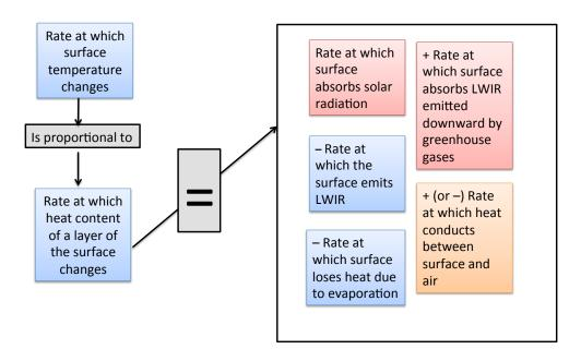
Using this relationship, we can calculate how fast the surface temperature changes and estimate temperature in the near future (at least, if the model is complete and accurate). We can run this more complete model, compare the results to observed daily temperature cycles, and see how well the model performs. That is, we can evaluate, or *validate*, the model.
