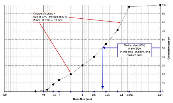
Now we need to plot a cumulative weight % vs. grain size on semi-log paper, as shown at left and demonstrated in class. Then, from the graph, you can determine the following two parameters.
