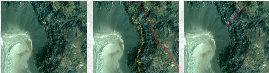
**3D visualization.** Computer graphics can help show the relationships of dipping sedimentary rocks, and can be adjusted interactively. The two images below show different views of the same area, and clearly demonstrate the eastward dips computed above.
