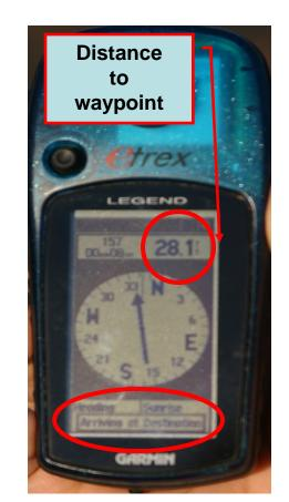
9. Use the Toggle Button to highlight 'GoTo' function, moving up/down or right/left
