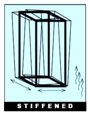
Shock and vibrations sent into and contained within stiffened frame.
