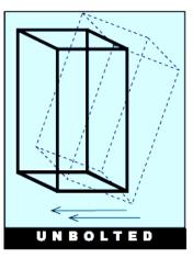
Reaction of a cabinet to seismic ground motion.
