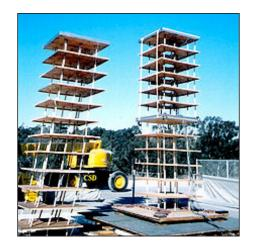
Base isolation, also known as seismic or base isolation system, is a collection of structural elements which should decouple a structure from the ground. If the ground below a building shifts abruptly to the left as shown in the experimental buildings here, the building with base isolation on the right becomes an inertial mass that stays in the same place during the jolt due to structural elements that decouple it from the earth.
