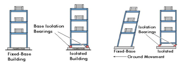
Movement of Building with Fixed-base Isolation and with Base Isolation
